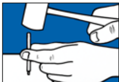
3. Tap the top of the tool with a small plastic hammer until the receptacle is seated at the proper height. The press ring keeps the receptacle in place.
